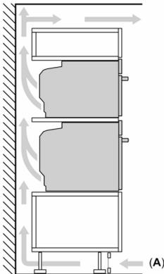
A: Dovod vazduha  $\geq 200 \text{ cm}^2$
