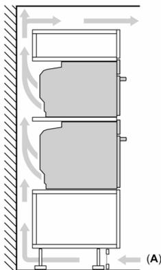
A: Dovod vazduha  $\geq 200 \text{ cm}^2$
