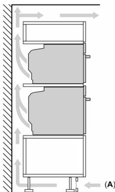
A: Dovod vazduha  $\geq 200 \text{ cm}^2$
