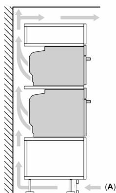
A: Dovod vazduha  $\geq 200 \text{ cm}^2$
