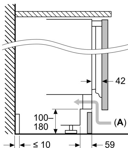
A: Dovod vazduha  $\geq 200 \text{ cm}^2$
