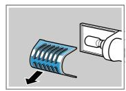
4. Replace the illuminant. Replacement illuminant: 220-240 V AC, E14 bulb holder, see the defective illuminant's wattage.
