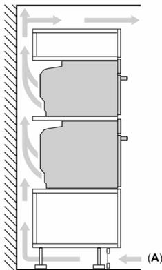
A: Dovod vazduha  $\geq 200 \text{ cm}^2$
