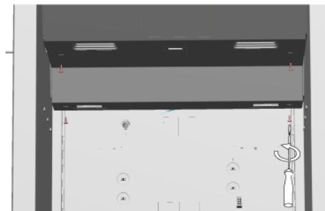
3. 1. Pull the evaporator cover horizontal direction to release it from clips (1).
